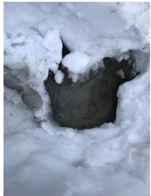
Exhibit 2-4: Water in MW-12-10 monument, overtopping the casing.
